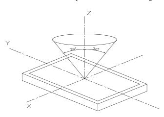
Inspection should be performed within angle  $\varphi(\phi)$  is usually 30°) from Z axis to each X and Y. Inspection distance in any direction within  $\varphi$  must be kept 30±5cm from the display surface.
