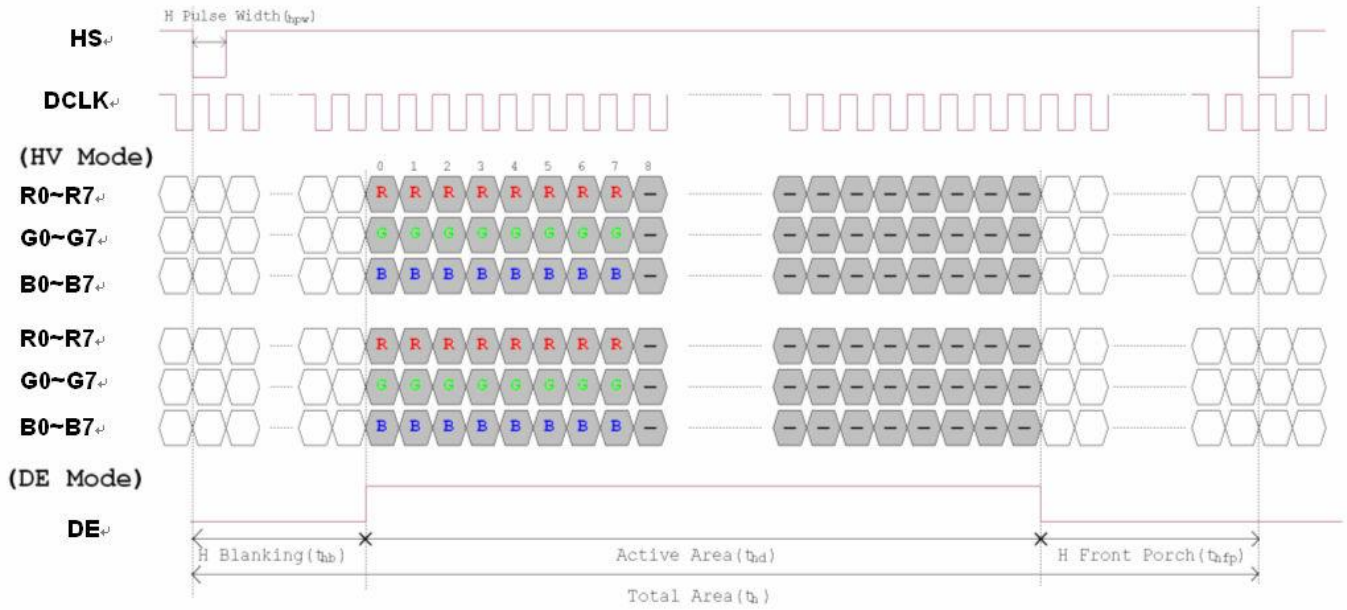
Figure 3. 1 Horizontal input timing diagram.
